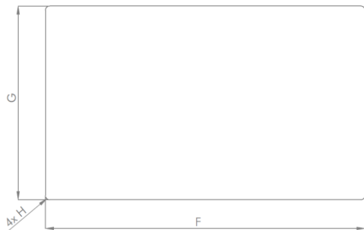
Illustration 24: Dimensions Open Frame Cutout Counterplate
